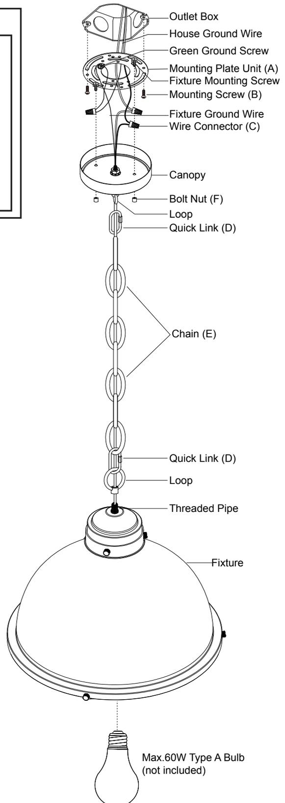
7. Attach the canopy to the mounting plate unit (A) and secure it with two bolt nuts (F) .
