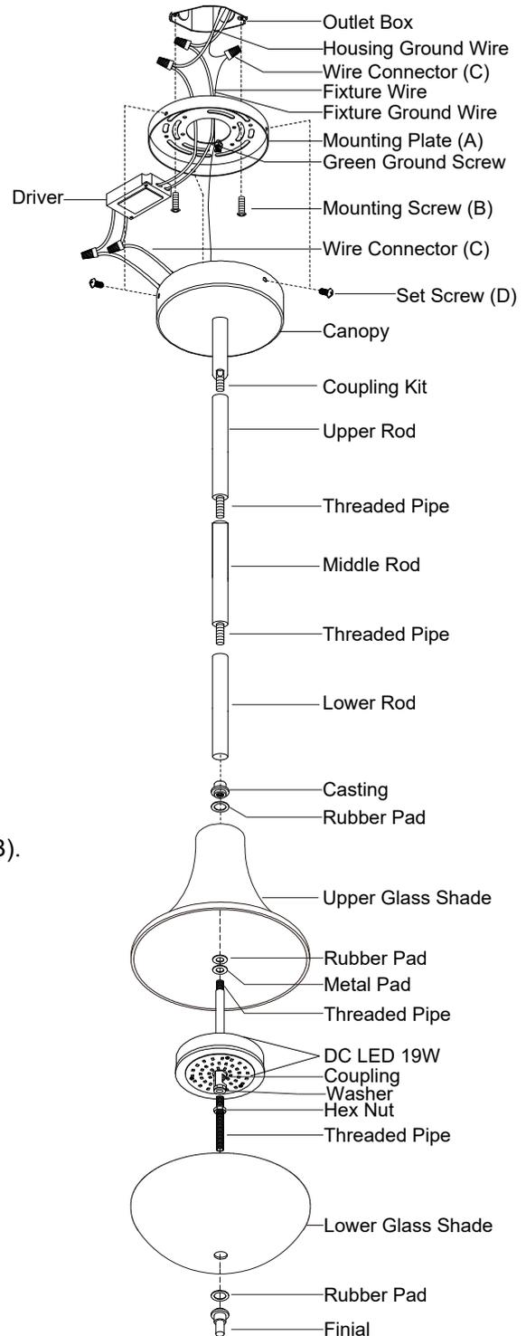
8. Pull out the source wires from the outlet box. Make wire connections using wire connectors (C) as follows:
